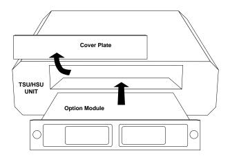
Figure 2-1. Installing the Option Module
